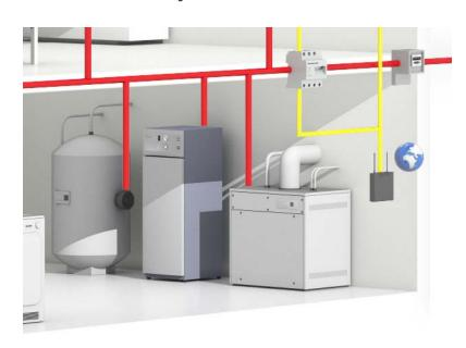
CHP plants are extremely suitable as controlled power generators in the scope of future intelligent energy management, since the heat they generate during operation can be ideally stored in tap and heating water.
