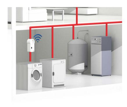
Electrical appliances that do not have specific turn-on times can be remotely activated by the Sunny Home Manager and are thus included in the intelligent load management system.
