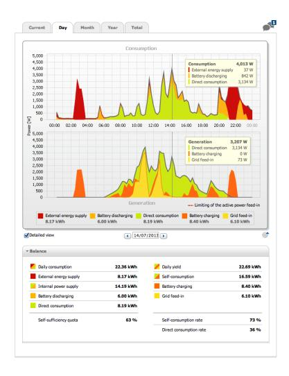
The analysis page displays the energy balance for the desired time period and facilitates a variety of analyses.
