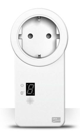
Loads that can be operated at various times and have no control interface can be activated at the optimal time by the Sunny Home Manager via an SMA radio-controlled socket. The socket also features an integrated measurement function that records the exact energy consumption of the connected device to improve planning accuracy.
