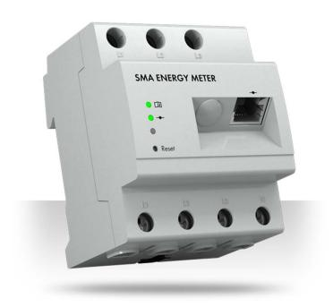
As a powerful measuring device for intelligent energy management, the SMA Energy Meter takes electrical measured values and communicates the data of purchased electricity and grid feed-in via Speedwire to the Sunny Home Manager or to the Sunny Boy Smart Energy.
