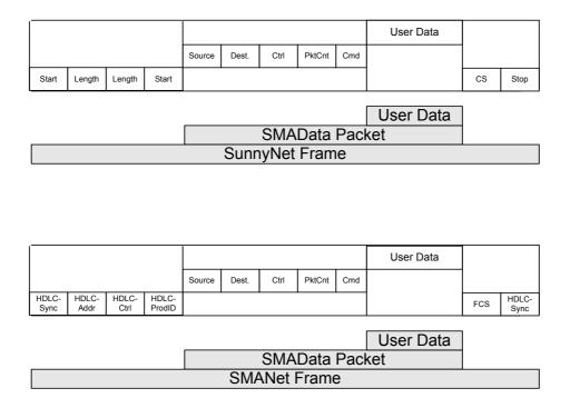
Figure 2: Packet Encapsulation of the SunnyNet and SMANet Telegram Frames
