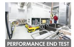
In the performance end test chambers, the inverters are tested in the effective V-loop procedure at 100% power.
