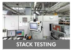
In contrast to other manufacturers, SMA develops and produces numerous modules itself. This includes printed circuit boards (PCBs), DC and AC modules and inverter stacks. SMA tests the functionality of these components before they are installed in the inverter to obtain precise information about their functionality in the same position they will be later in the inverter.
